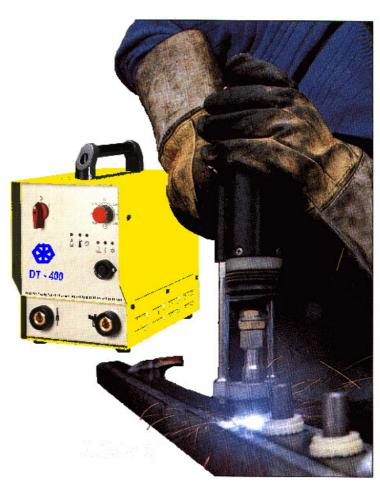
CNC/PC-controlled capacitor stud welding unit. Capacity 1-8 mm on sheet metal, welds up to 60 threaded studs per minute.
